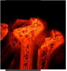
Hot forging gives the shape to our adjustable wrenches. Our high tonnage forging hammers provide us total independence and control of the process.
