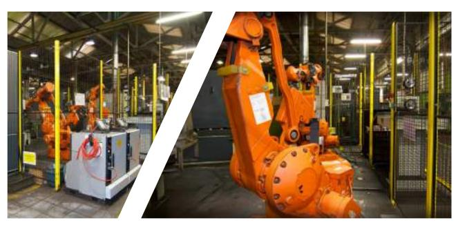
We have robotized facilities to complete the whole grinding processes of our wrenches.
