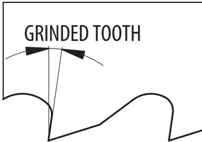
**Application:** for cutting common types of steels with a tensile strength up to 1700 N/mm<sup>2</sup>
