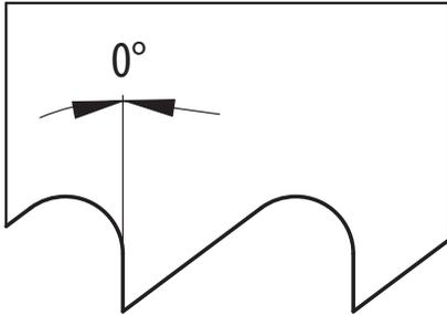
**Application:** for cutting common types of steels with a tensile strength up to 1400 N/mm<sup>2</sup>
