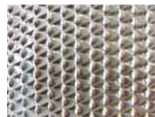
Milled Straight Cut with Chipbreaker
