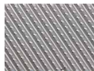
Milled Straight Cut with Chipbreaker
